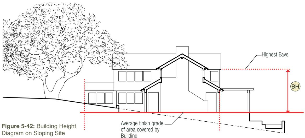
Figure 5-42: Building Height Diagram on Sloping Site
