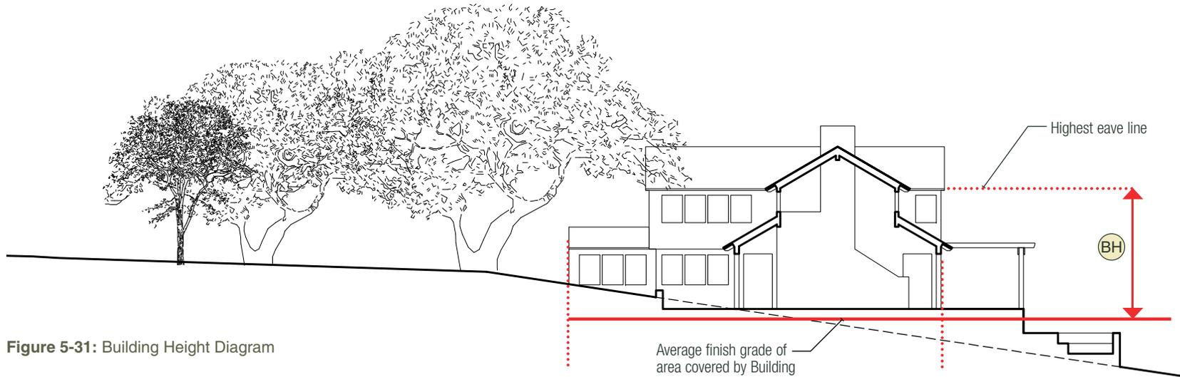
Figure 5-31: Building Height Diagram
