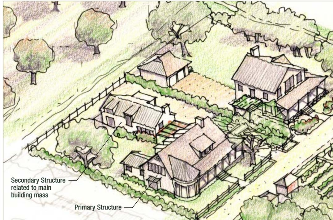
Figure 5-37: Massing Diagram
