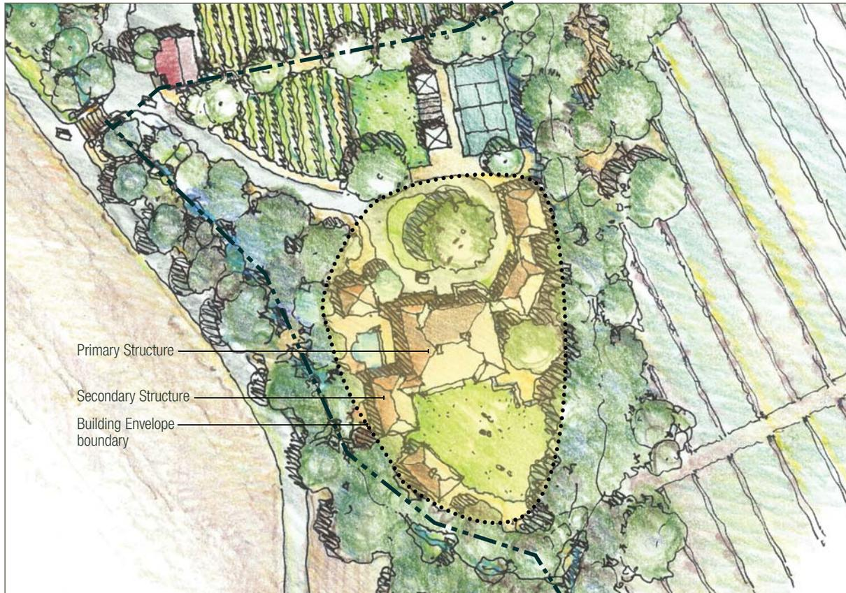
Figure 5-34: Compound Building Envelope Diagram
