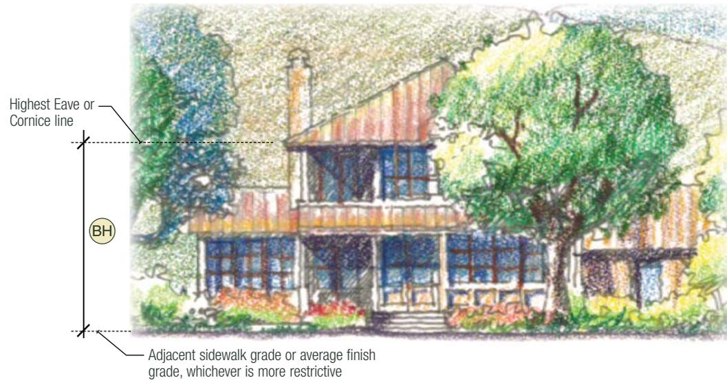
Figure 5-41: Building Height Diagram on gently sloping site
