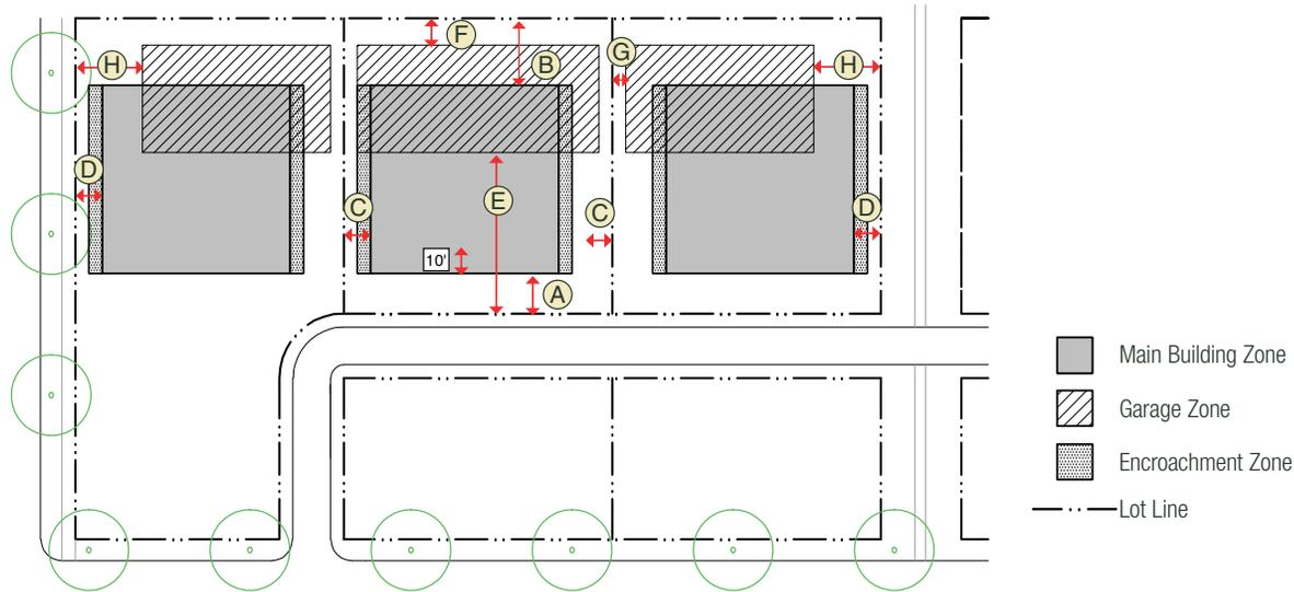
Figure 5-23: Building Placement Diagram
