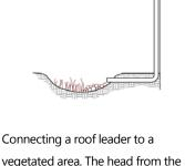
connecting a roof leader to a vegetated area. The head from the eave height makes it possible to route roof drainage some distance away from the building.
